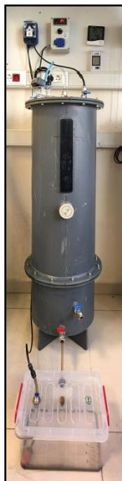
Figure 2. Anaerobic landfill bioreactor used in this study
