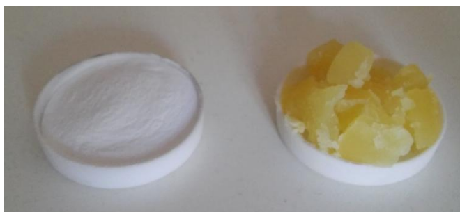
Figure 5. The magnesol absorbent before and after the purification process
