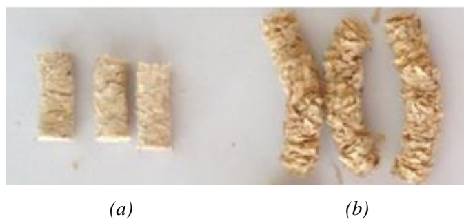
Figure 5. The bio-pellets: (a) G0 pellets, (b) G25 pellets
