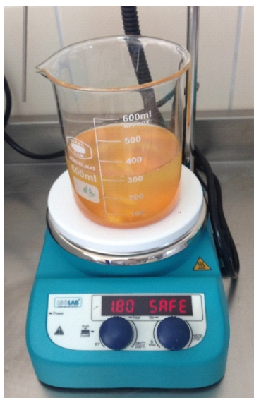
Figure 1. Fenton Process System
