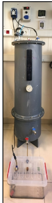
Figure 2. Anaerobic landfill bioreactor used in this study
