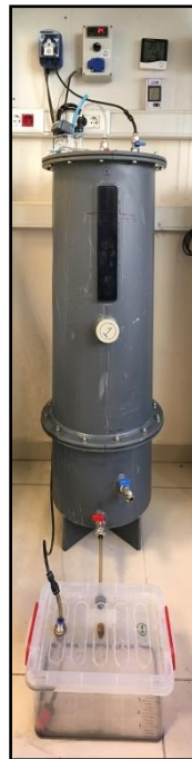
Figure 2. Anaerobic landfill bioreactor used in this study
