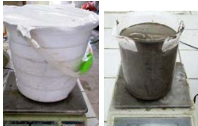
Figure 2. (a) Checking density of the foam, (b) and mortar.
