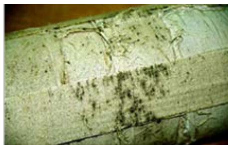
Figure 6. Influence of moisture on bag for propellant charge ammunition 155mm [8]
