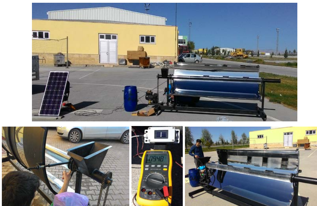
Figure 2. Parabolic through solar drying system and its components using for experimental study
