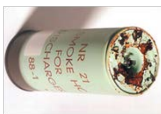
Figure 12. Corrosion caused by moisture on pyrotechnical materials in ammunition [5]
