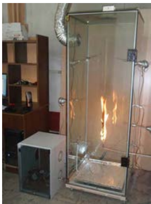
Figure 1. The appearance of test machine and the sample burning [15]
