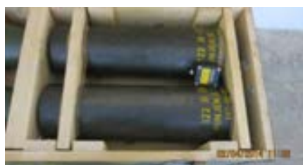
Figure 14. Wooden box with ammunition without internal packing (Eastern concept)
