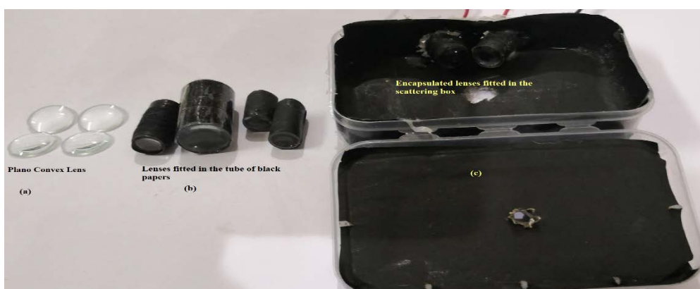
Figure 7. Image of (a) Plano-convex lens (b) Lenses fitted in the paper tube (c) Lenses encapsulated in a scattering box
