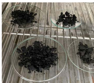
Figure 1. The Dried Alkali-Modified Fly Ash/Fe 3 O 4 /CuO catalyst
