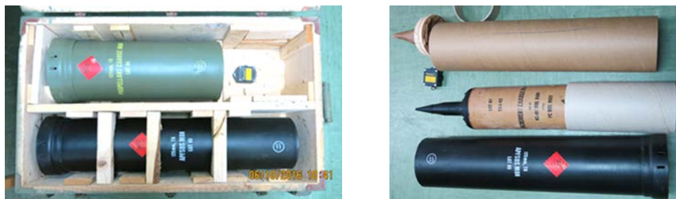
Figure 7. Tank ammunition 125 mm APFSDS-T M88, packing
