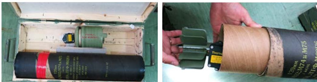
Figure 5. Mortar ammunition 120 mm M62, packing
