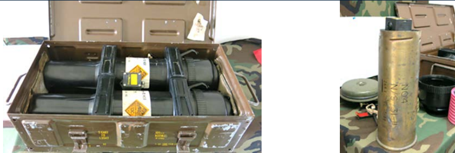
Figure 3. Cartridge propelling 105 mm L35, packing
