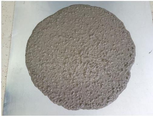
Figure 3. (a) Mixture S5 – slump-flow
