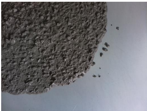
Figure 2. (a) Mixture S10 – slump-flow
