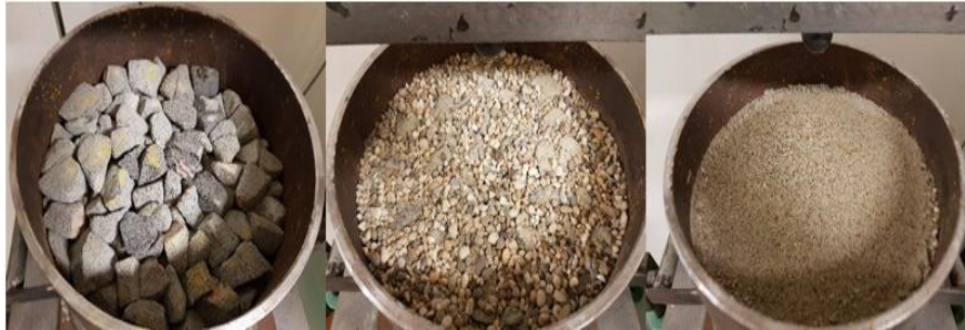
Figure 2. Foam glass aggregate laboratory sample preparation (left to right: foam glass aggregate, with gravel layer, sand load distribution layer)
