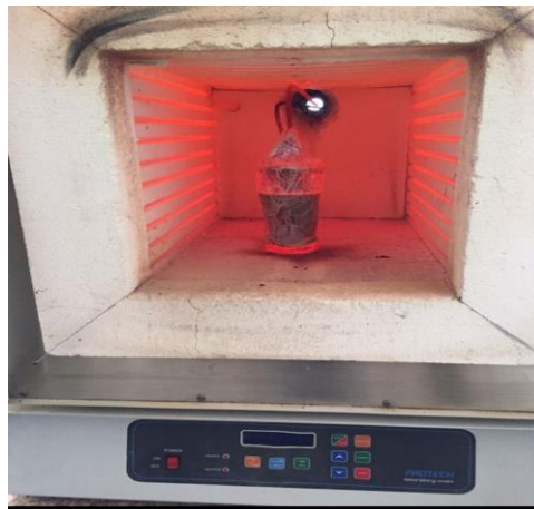
Figure 1. Reactor and muffle furnace for pyrolysis experiments
