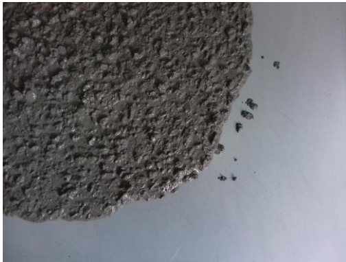
Figure 2. (a) Mixture S10 – slump-flow
