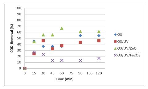
Figure 7. The effects of ozone based oxidation processes on COD removal for BPA treatment
