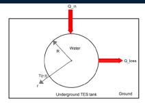
Figure 3. The energy balance of the underground TES tank.
