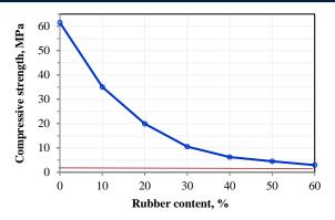
Figure 4. Effect of rubber content on compressive strength
