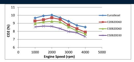
Fig.6. Change of CO2 according to engine revolution
