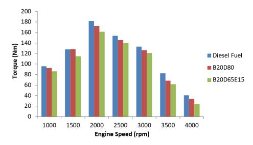
Figure 3. Variation of engine torque with engine speed
