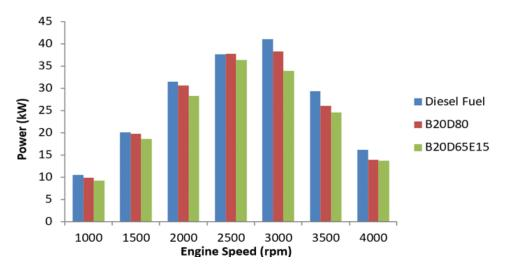
Figure 2. Variation of engine power with engine speed
