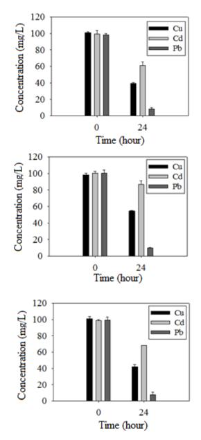
Figure 3. The effect of changing A/C ratio on heavy metal adsorption from a synthetic wastewater (a) (1g/1g); (b) (1g/2g); (c) (2g/1g).
