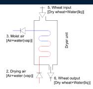
Figure 2. Schematic of dryer unit.
