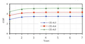
Figure 8. Effect of CE on COP of the heat pump (limestone,  $Ac = 30 \text{ m}^2$ ,  $V = 200 \text{ m}^3$ ,  $W_5 = 20 \text{ kg/hr}$ ).
