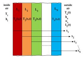
Figure 2. Schematic view of a multilayer wall.
