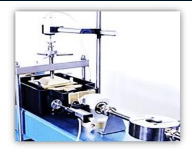
Figure 9. Direct shear test machine
