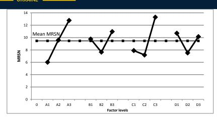
Figure 14. Effect of factor levels on S/N ratio
