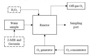
Figure 17. Schematic diagram of the experimental set-up.
