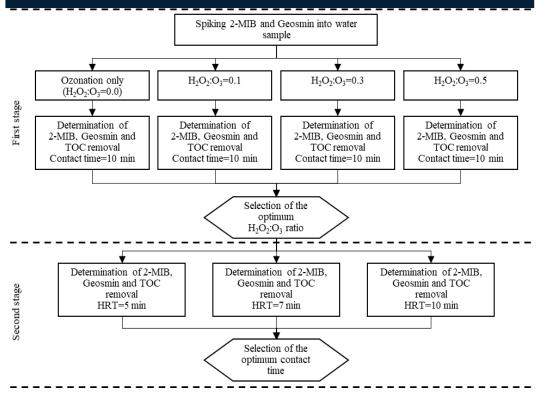
Figure 18. Schematic diagram of the experimental plan.
