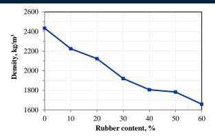
Figure 6. Effect of rubber content on the density.
