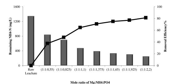
Fig.2 Ammonia removal efficiencies for the MAP precipitation experiment in which the PO4-P ratios were increased
