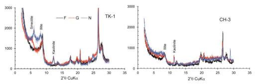
Figure 3. Representative X-ray diffraction pattern of <2 \mu m fraction oriented in natural condition (N), after heated at 490  $^{\circ}C(F)$  and solvated in ethylene glycol atmosphere (G).
