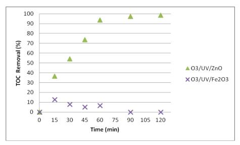
Figure 6. The effects of photocatalytic ozone processes on TOC removal for BPA treatment
