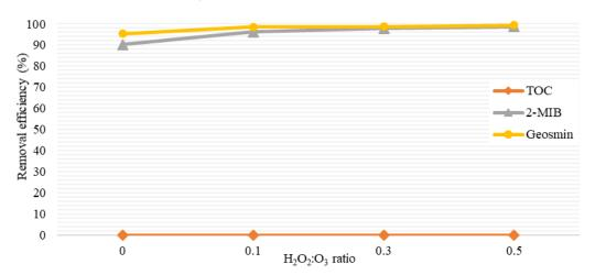
Figure 20. Removal efficiencies of TOC, 2-MIB and geosmin at different H<sub>2</sub>O<sub>2</sub>:O<sub>3</sub> ratios (contact time: 10 min).
