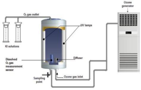
Figure 2. Ozone reactor system.
