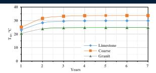
Figure 4. variation of the TES tank temperature for September (Ac=30  $m^2$ , CE=40%, V=200  $m^3$ , W5=20 kg/hr)
