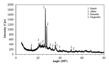
Figure 1. X-ray diffractogram of fly ash
