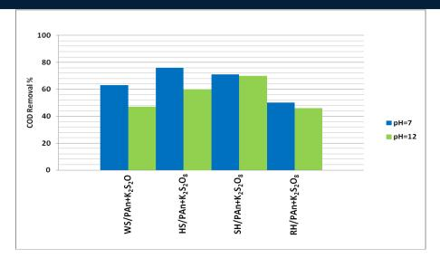
Figure 3. The effect of adsorbent on the COD removal yields (100 mL of Laundry wastewater, 1g of adsorbent amount, 120 min reaction time, 150 rpm stirring rate).
