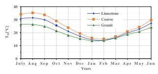
Figure 6. Effect of earth type on water temperature in the TES tank during fifth year of operation
