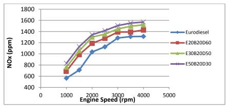
Fig.8. NOx change according to engine speed
