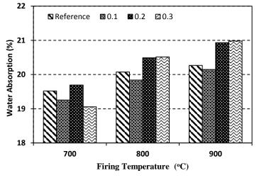
Figure 2. Water Absorption of Specimens
