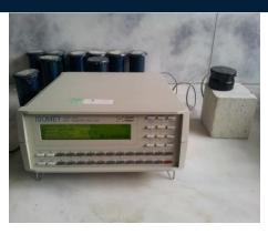
Figure 1. The thermal property measurement device used in the study (TS EN 12667)
