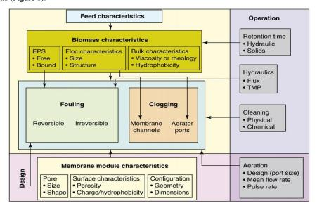
Figure 15. Interrelationship between MBR parameters and fouling [2]
