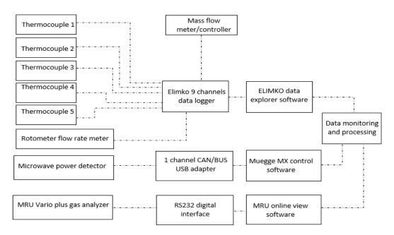
Figure 3. The measurement and data acquisition chain
