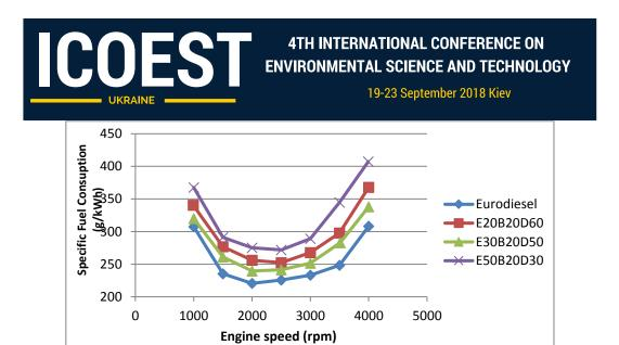
Fig. 4. Exchange of specific fuel consumption values according to engine RPM
