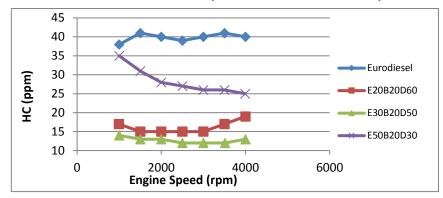
Fig.7. Change of HC according to engine speed
