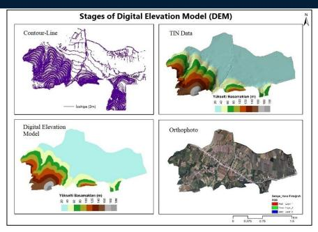
Figure 3 Digital Elevation Model And Orthophoto
