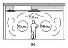
Figure 2. Mechanical ventilation application. A) displacement ventilation, b) mixing ventilation [10].
