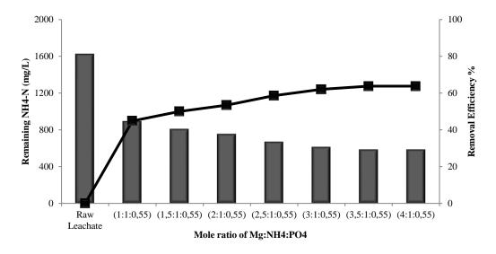
Fig. 1. Ammonia removal efficiencies for the MAP precipitation experiment in which the Mg ratios were increased
