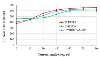
Figure 10: Effect of current direction on near field dilution in summer conditions
