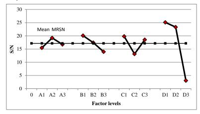
Figure 13. Effect of factor levels on S/N ratio
