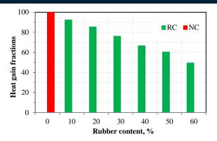
Figure 8. The percentages of max. heat gain fractions for each south-wall construction with different rubber ratios.
