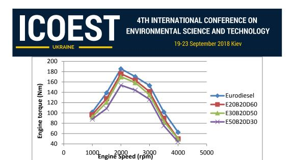
Fig. 2. Engine torque values according to engine RPM
