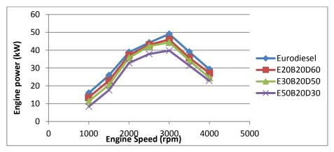
Fig. 3. Engine power values according to engine RPM
