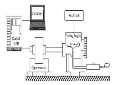
Figure 1 Schematic view of the Motor Test Assembly
