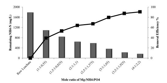
Fig.3. Ammonia removal efficiencies for the experiment of MAP precipitation, in which both Mg and PO4-P ratios were increased
