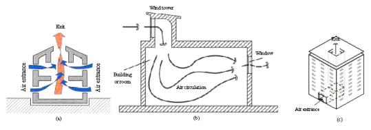
$Figure\ 1.\ Fresh\ air\ intake\ applications\ in\ natural\ ventilation\ [6].$
