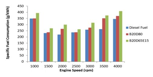
Figure 4. Relationship between specific fuel consumption and engine speed
