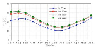
Fig. 5. Variation of the TES tank temperature with years (limestone,  $Ac = 30 \text{ m}^2$ , CE = 40%,  $V = 200 \text{ m}^3$ ,  $W_5 = 20 \text{ kg/hr}$ ).
