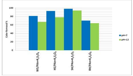
Figure 1. The effect of adsorbent on color removal yields (100 mL of Laundry wastewater, 1g of adsorbent amount, 120 min reaction time, 150 rpm stirring rate).
