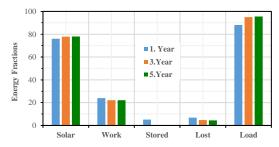
Figure 11. Variation of energy fractions with years (limestone,  $Ac=30 \text{ m}^2$ , CE=40%,  $V=200 \text{ m}^3$ ,  $W_5=20 \text{ kg/hr}$ ).
