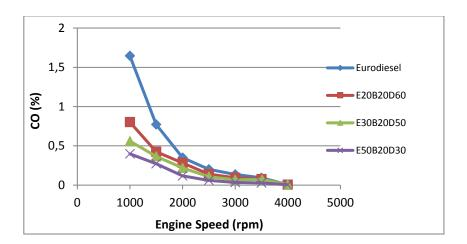
Fig.5. CO changes depending on engine speed
