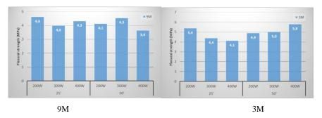
Figure 5. The flexural strength of mortars
