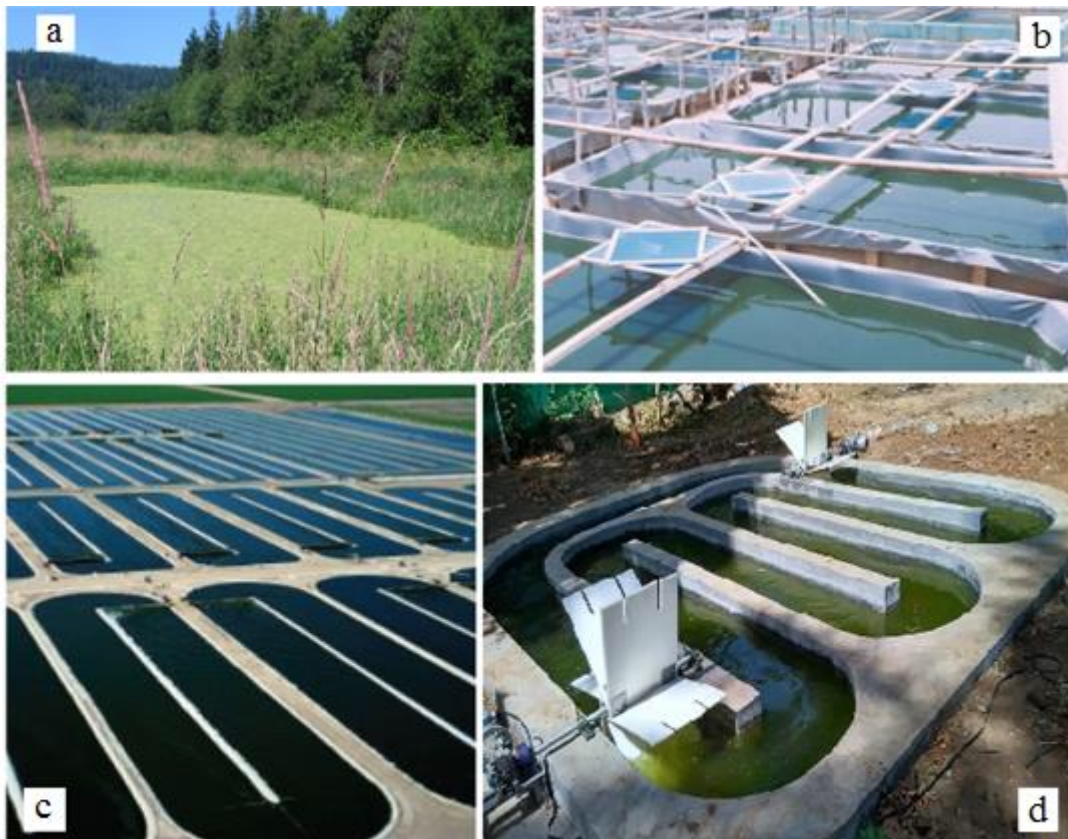
Figure 5. Different designed open pond systems [21]
