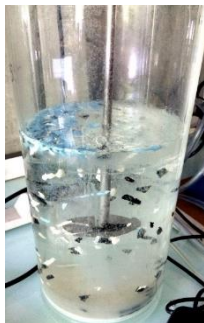
Img.1 Self designed glass flotation column
