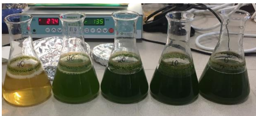
Figure 1. The experimental setup of microalgae treatment to baker's yeast manufacturing process wastewater.
