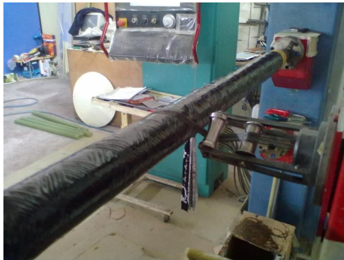
Figure 1. Production of CNT reinforced nanocomposite tubes by filament winding method (23).
