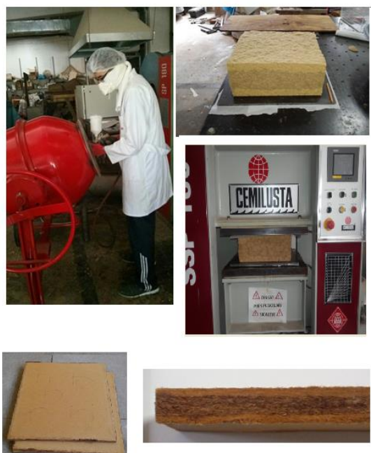
Figure 2. Production of three-layer MDF panels at the laboratory
