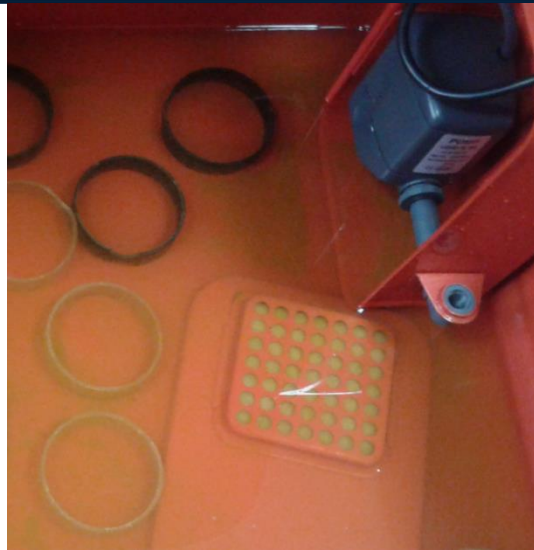
Figure 2. CNT-reinforced test specimens immersed in seawater
