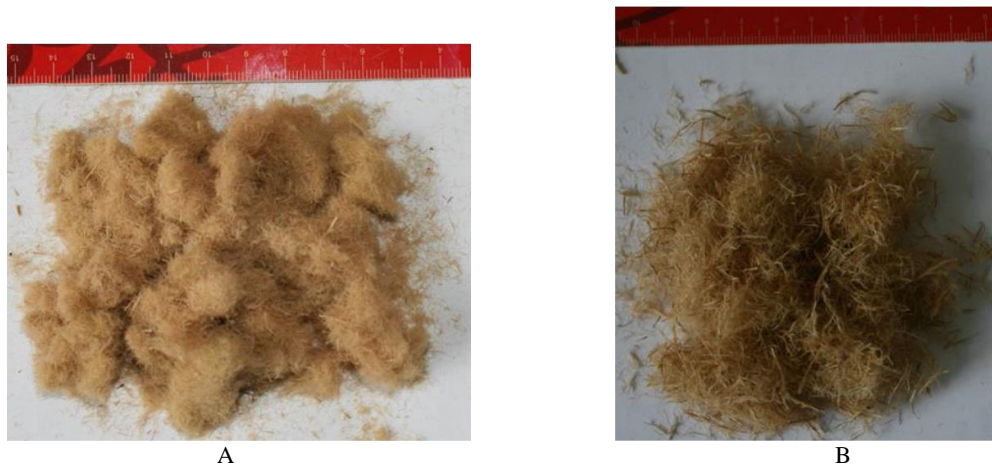
Figure 1. A: Fine wood fibers (pine) in face layers of MDF. B: Coarse wood fibers (beech) in core layer.
