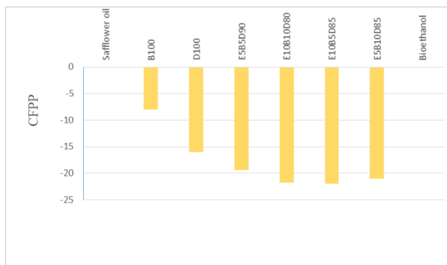
Figure 12. Cold filter plugging point values of the fuels
